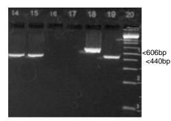
Wells 14 and 15 are homozygous for the mutant allele. Wells 16 and 17 are blanks. Well 18 is a WT control and Well 19 is a homozygous control. Well 20 is 1Kb+ Ladder (Invitrogen Cat# 10787-018).
